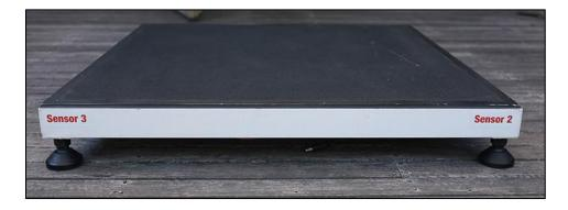
When using the InnerBalance software it is crucial that you enter the force plate from the 'front of the platform' and face the rear of the platform. (Refer below) It will then read the Medio-Lateral (ML) and Anterior-Posterior (AP) data correctly!
