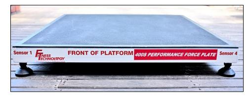
The opposite side of the force plate will be labelled with Sensor 3 (LC3) and Sensor 2 (LC2). This is what we refer to as the rear of the force plate. (Refer below)
